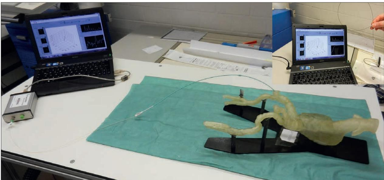
Figure 3: Experimental navigation in a 3D-printed model using fiber-Bragg-technology (Fiberoptic 3D-Shape System, Photonic Concepts, Goslar, Germany)
